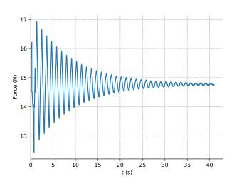
We want to be sure that the amplitude of the oscillations is small enough when we measure the period (to avoid nonlinearity of springs). We find
